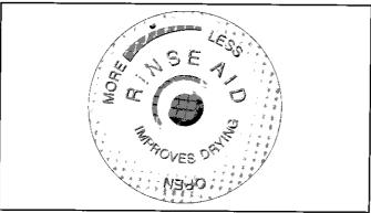
To add rinse aid to the dispenser, turn the cap counterclockwise to open. Remove the cap and pour liquid rinse aid into the opening. Replace the cap and turn it clockwise.
