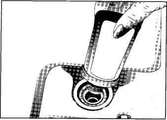
An adjustable cap found on some models allows you to adjust the amount of rinse aid dispensed. A raised dot on the cap indicates the recommended initial setting. Typically, use the LESS setting for soft water and the MORE setting for hard water. Set the cap anywhere between these amounts as needed. To improve drying, turn the cap towards the MORE setting. When adjusting or replacing the cap, be sure it is securely in place before closing the dishwasher door.
